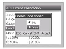
**Step 3.** When both the timers have been set you are able to 'Enable Load Shed' at the 'Load shed' function.
