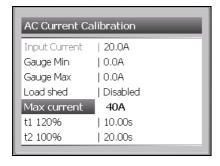
The Load shed current has two timers the first one of which to expire will activate the Load shed relay output.
