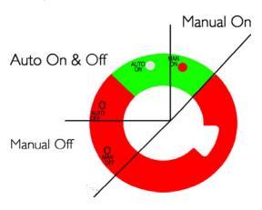
**Auto Operation:** The 701-MD moves from a state of "Auto Off" to "Auto On" when the remotely mounted switch is turned on. During the time that the battery switch is in "Auto On" mode, the "Auto On" LED is illuminated.
