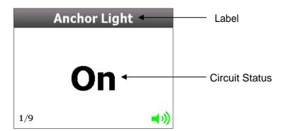
The systems in operation functions of this meter can be used to monitor essential circuits and inform the skipper about the circuit's state. Up to 8 inputs can be used as Systems Operation and they can all be displayed on the Mimic page for quick reference.
