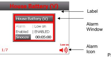
When an alarm is active you will see an Alarm Window for each active alarm and the buzzer/external alarm will sound. The Alarm Window will tell you which input is alarming and what type of alarm it is i.e. Low On or Low Voltage. The label for all alarming circuits will be red also.
