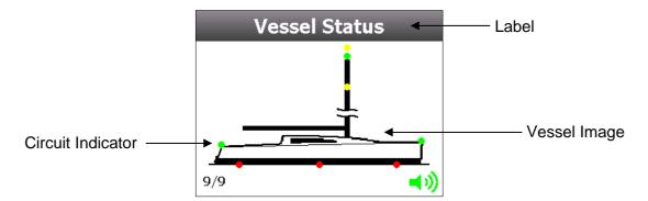
The Mimic page will give the user a view of all systems in operation circuits on a selectable boat image. The 5 default boat images can be chosen from the following:
