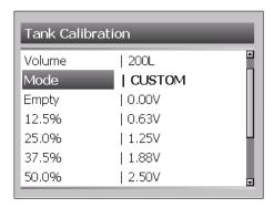
Use custom mode if the set point voltage values are already known from a previous tank meter setup. They can be directly entered without any other calculations.
