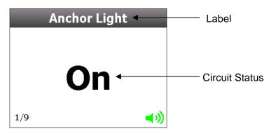
The systems in operation functions of this meter can be used to monitor essential circuits and inform the skipper about the circuit's state. Up to 8 inputs can be used as Systems Operation and they can all be displayed on the Mimic page for quick reference.
