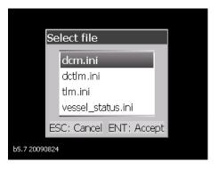
When first powering up the DCSM the user will be presented with a group of default meter file types to choose from. The table below shows the 4 Default Meter Types with an X showing what inputs are enabled. Please select the Meter Type that is closest to your application:
