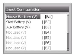
Press Enter on the input you would like to configure. The input settings will vary depending on what type of Input you are using.
